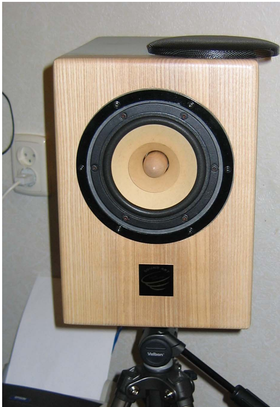
SFR145-8 fullrange loudspeaker, back loaded horn application
