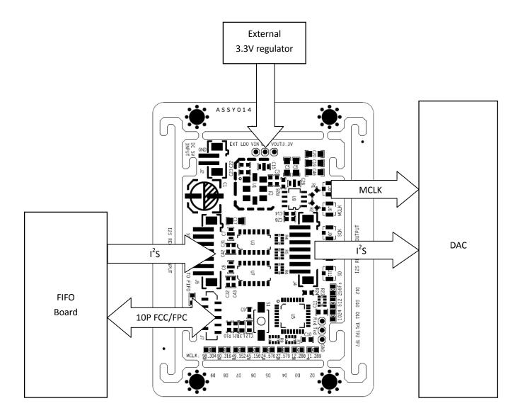
In this configuration, the Si570 Clock Board is used without an isolator board. The Si570 is connected directly to the FIFO board by a 10P FFC/FPC cable and obtains its power from the FIFO board. In this configuration, the Si570 Clock Board requires an external 3.3V regulator. Appropriate regulators are discussed below.
