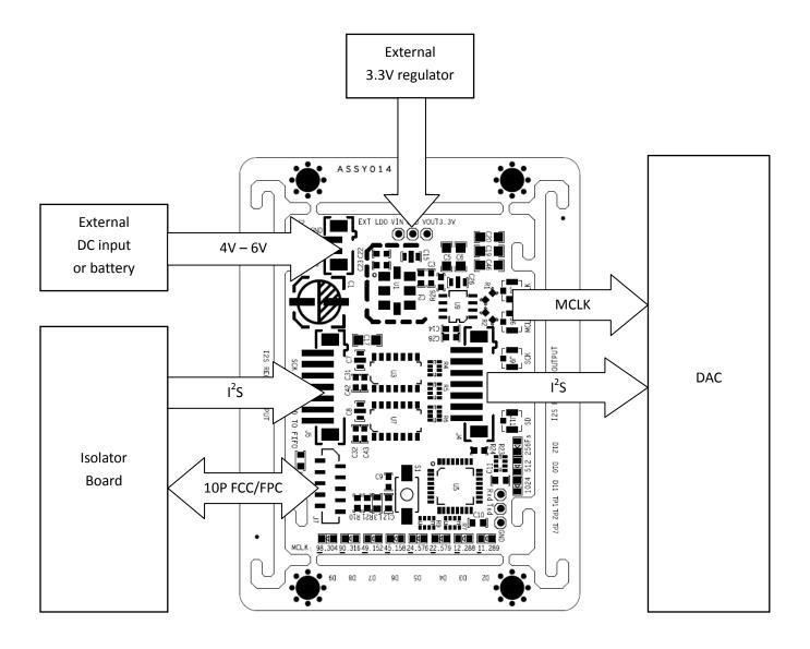
This is the recommended, "full feature" configuration. The Si570 Clock Board is isolated from the I<sup>2</sup>S source and FIFO by the isolator board (available separately). This isolation requires the Si570 Clock Board to have its own power source. Appropriate power sources are discussed below. Depending on the power source, the Si570 Clock Board may need an external 3.3V regulator. Appropriate regulators are discussed below.
