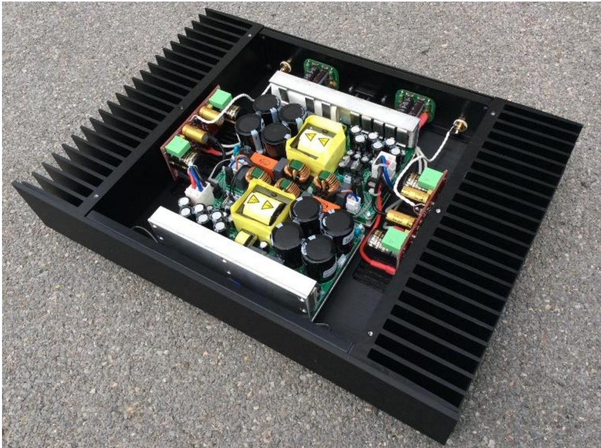
Prototype power amplifier showing dual mono power supplies.
