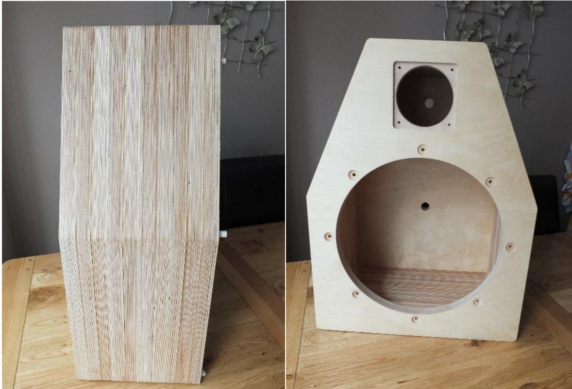
Laminated plywood construction provides an inert & elegant solution.
