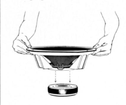
When the three screws are removed, carefully lift the magnet structure vertically from the basket assembly and flip structure over with the gap up.
