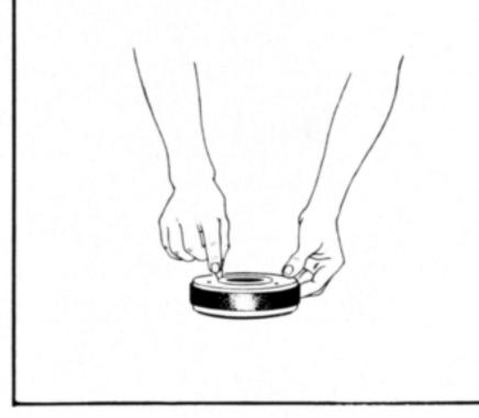
With the speaker face down, replace the three screws and tighten.
