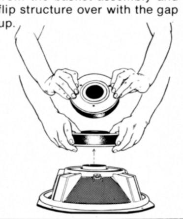
Firmly grasp both the basket assembly and the magnet structure with both hands and carefully turn the entire assembly over on its face.
