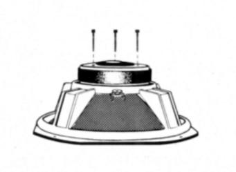
Place the magnet structure on a flat surface with the "gap" facing upward and carefully lower the new basket assembly onto the magnet structure. Use extreme care in order to avoid damaging the voice coil.
